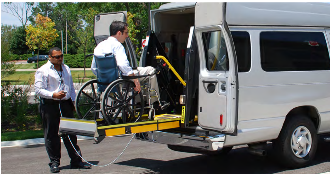
A wheelchair lift in operation.
