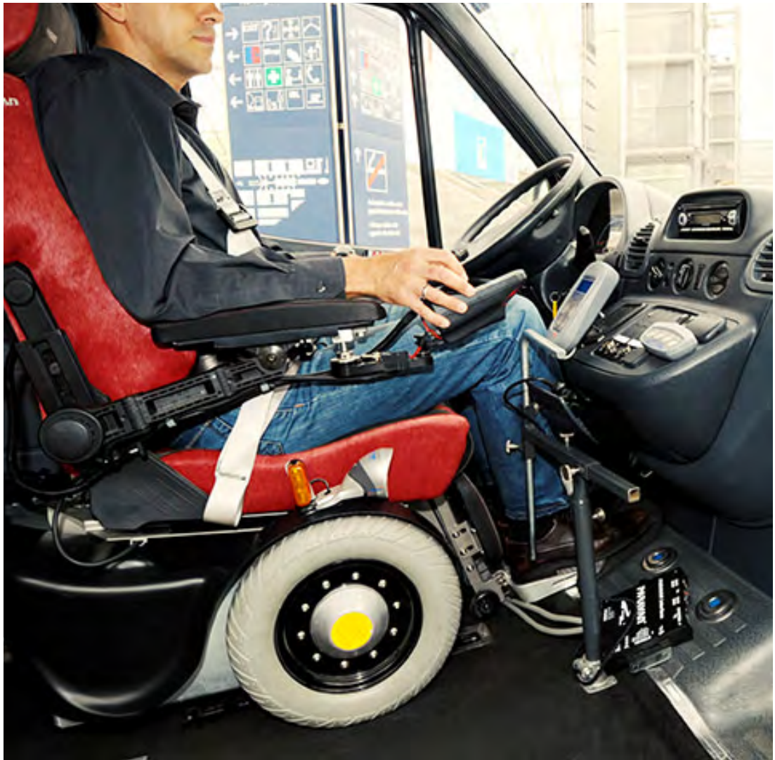
An example of a wheelchair accessible vehicle equipped with adaptive driving devices.
